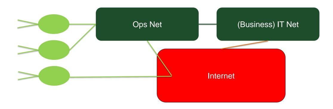
Ops Net: Manages operational assets using SCADA, directly and over TCP. Also has both internal network and tunnels over the larger Internet to various assets. Run by Ops team.
